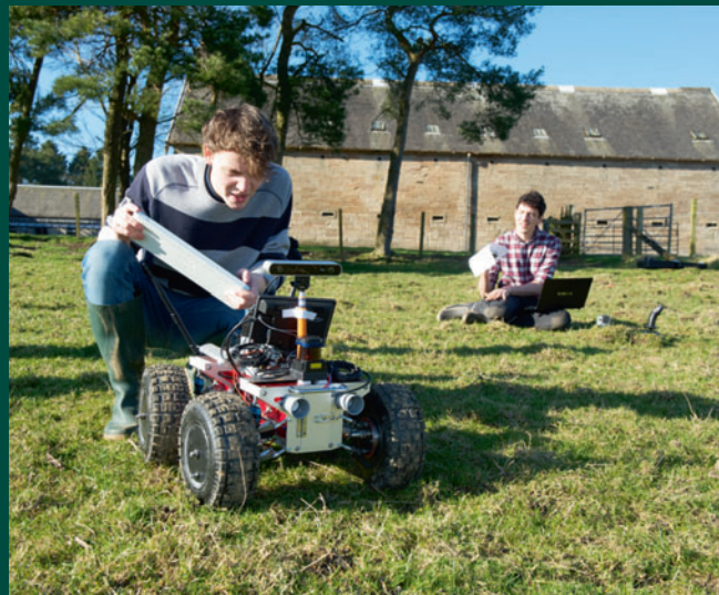
AgriRover consists of a mobile rover platform with a robotic arm that carries a soil sensing instrument. (Photo: University of Strathclyde)
